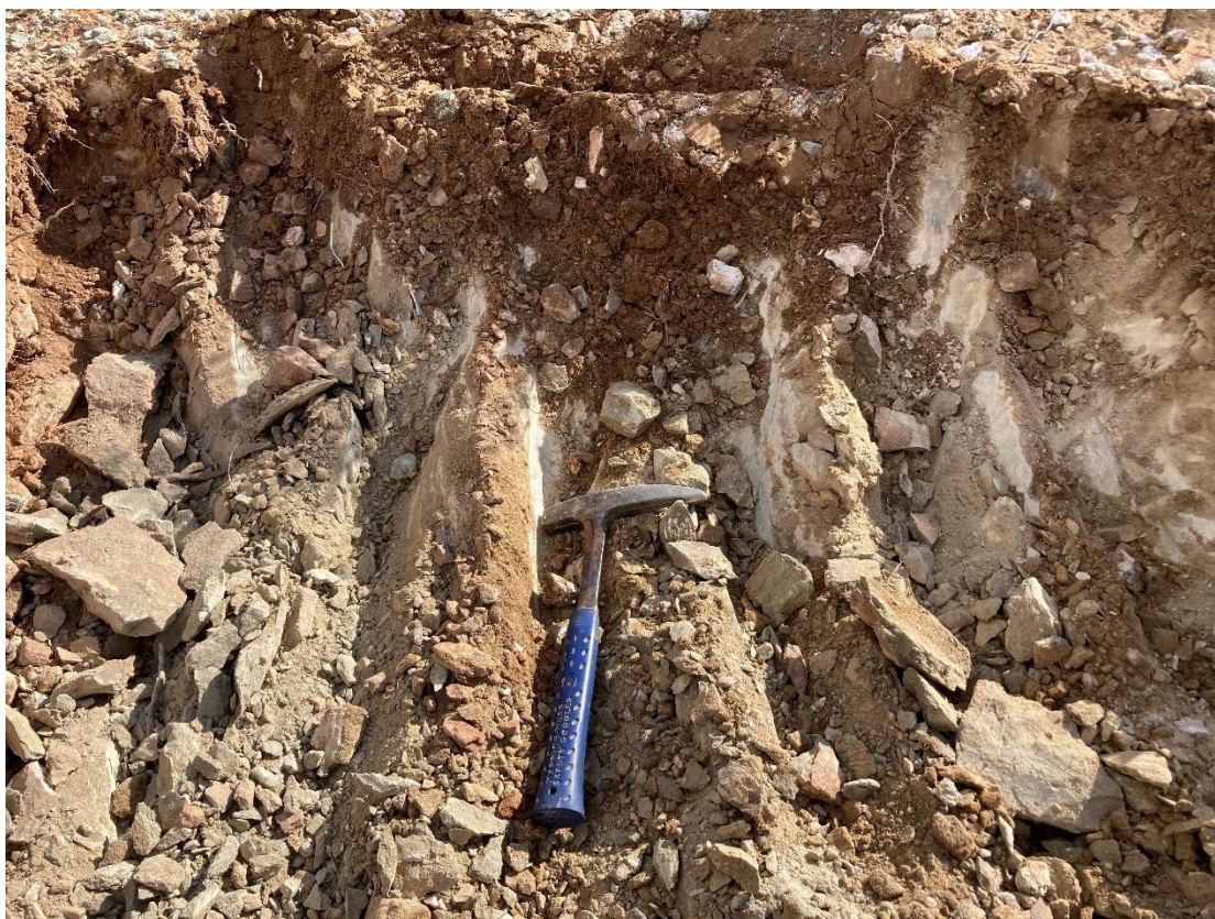
Figure 28 SMTP14 moderately weathered, medium hard rock, tillite
