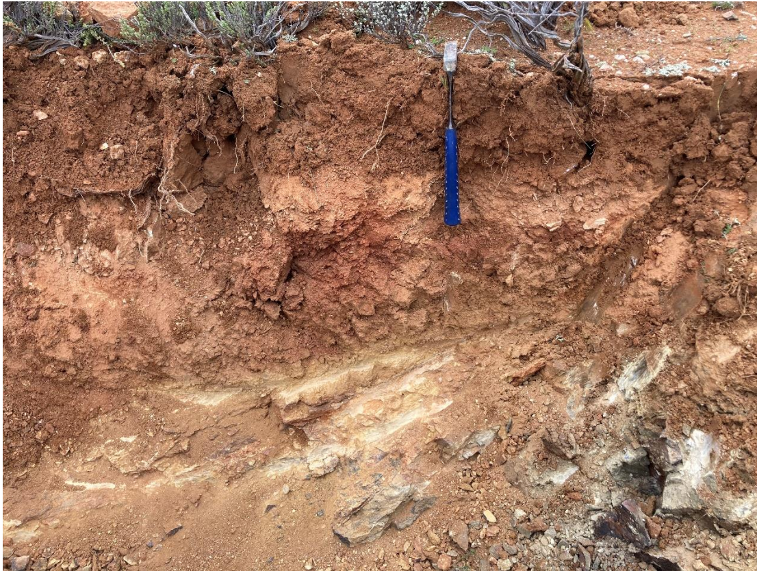
Figure 45 SMTP23 test pit profile
