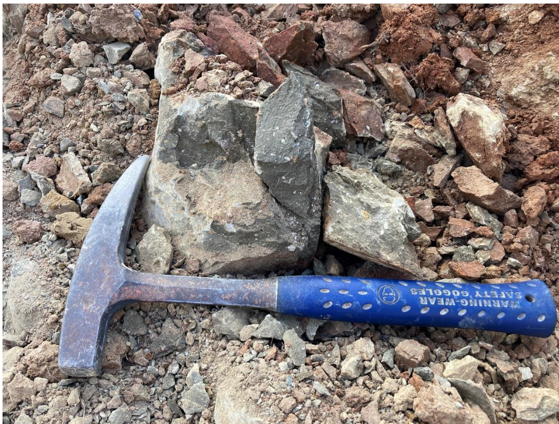
Figure 36 SMTP18 closeup of moderately weathered, medium hard rock, tillite
