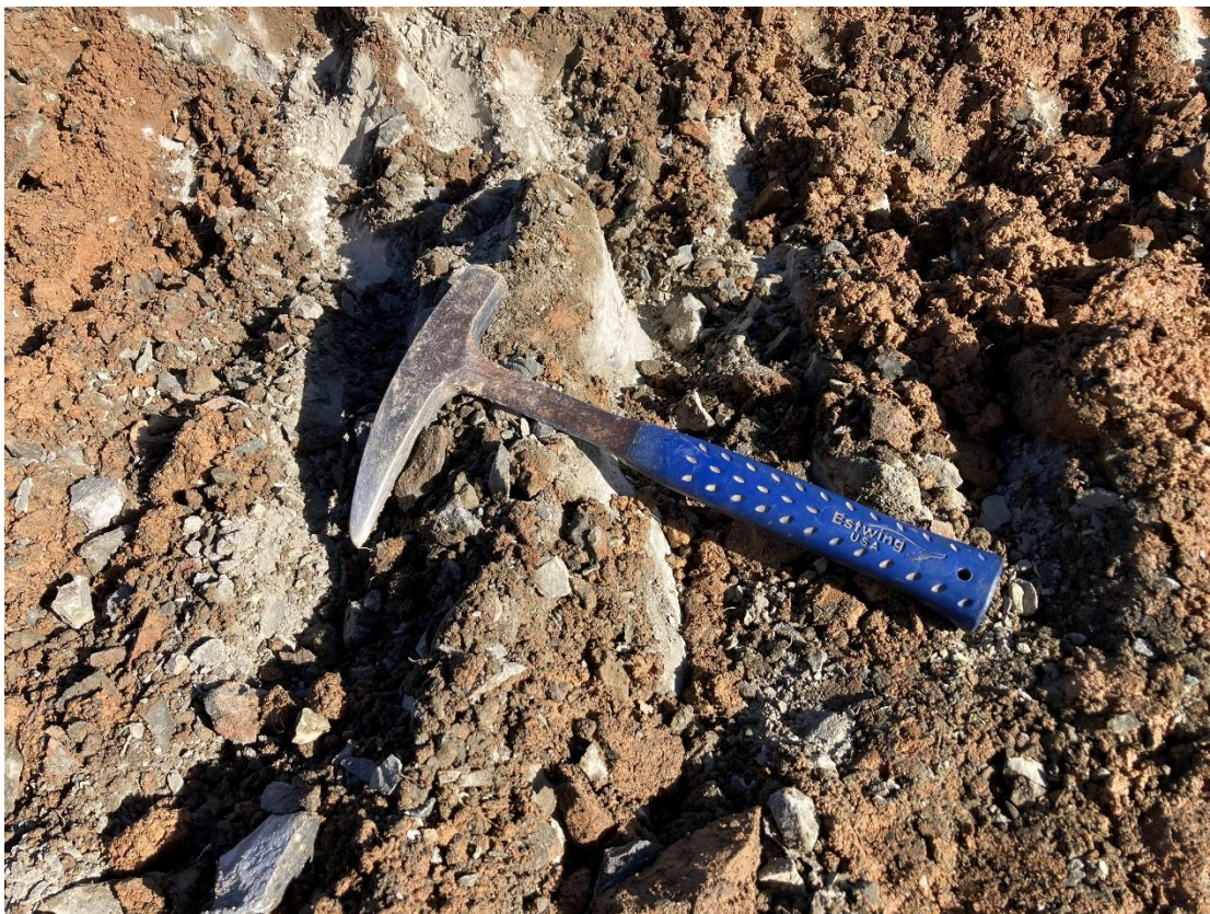
Figure 4 SMTP02 closeup of moderately weathered, medium hard rock, tillite
