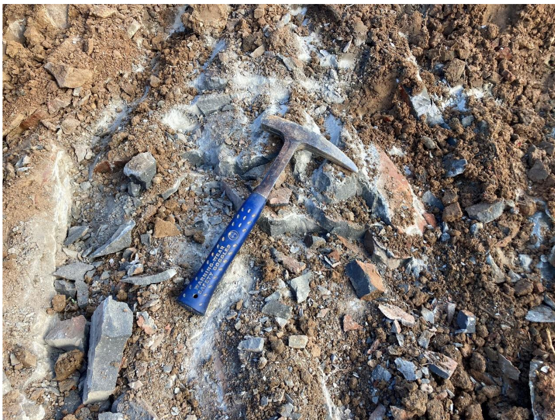
Figure 6 SMTP03 closeup of moderately weathered, medium hard rock, tillite
