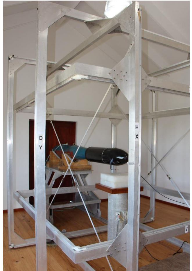
Figure 1: SANSa operates the only large tri-axial Helmholtz Coil system in Africa. The system can create or cancel any geomagnetic field and is used to evaluate and calibrate various magnetic sensors and magnetic systems prior to being integrated onto dynamic platforms such as satellites and UAVs.
