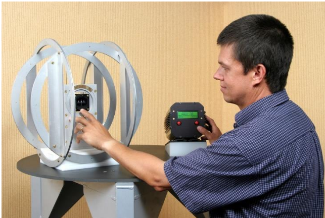
Figure 2: SANSa developed and designed a Magnetic Test Bench which is used for verification of standby (emergency) compasses prior to installation aboard aircraft. The system won several local and international design awards and is used extensively by the SA Air Force.
