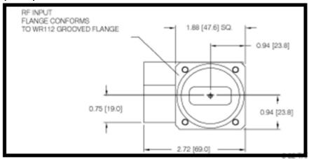
Input connector: Waveguide
